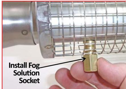
**Install Fog Solution Socket sent with the Water Conversion Kit. Snug with 14mm wrench.**
