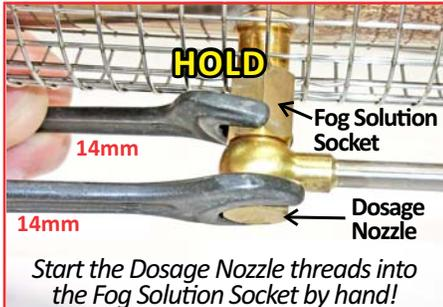
**Use one 14mm wrench to hold the Solution Socket & another to tighten the Dosage Nozzle.**
