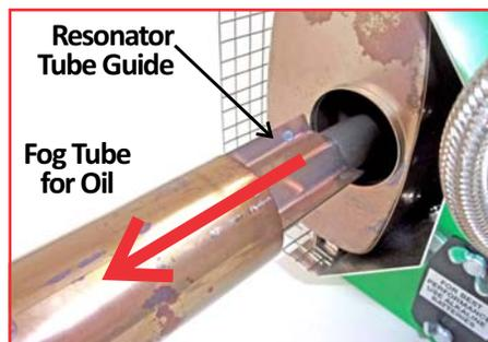
Remove the Fog Tube for Oil. It may bind on the Resonator Tube Guide, so twist while removing.
