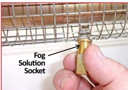
Loosen then remove the Fog Solution Socket. This will free the Protective Wire Guard.
